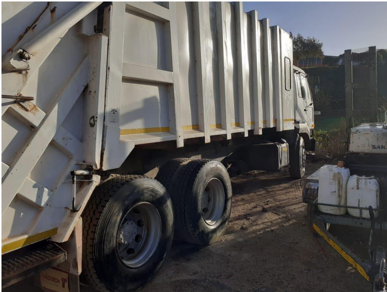
Figure 22: 19m 3 REL used in Caledon
